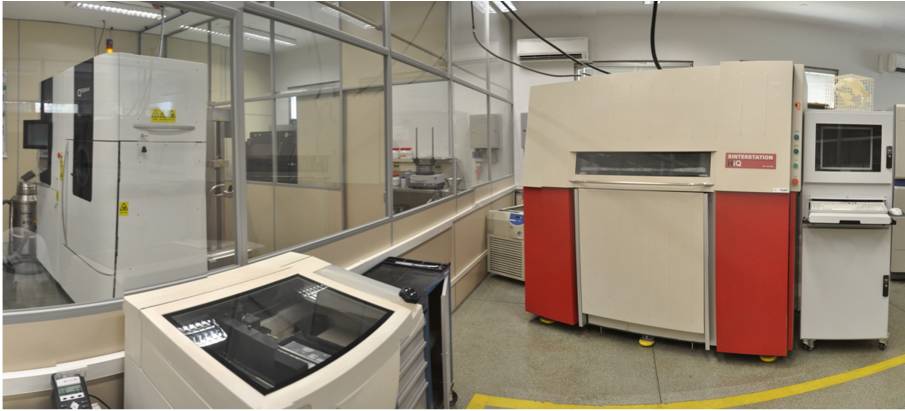
Fig. 1. Panoramic picture taken inside LAprint depicting EBM and SLS AM equipment. Available at [4]
