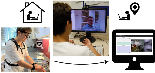
Fig. 1. Patients were equipped with a system to record their therapy sessions in their home environment. The data was streamed to the therapist UI, where the therapist had access to the egocentric video including gaze estimation and physiological measures. All icons are attributed to Flaticon.com
