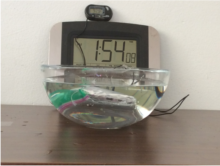
Fig. 6. Smartphone submerged in water bowl with an aquarium thermometer to monitor the water of the temperature.
