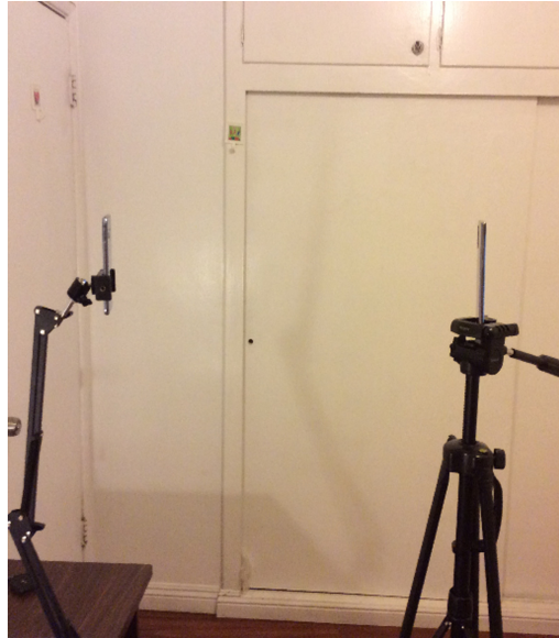
Fig. 9. Two smart phones are setup to face one another so that the WiFi adapter have direct access. This orientation is found to have the clearest signal reception.
