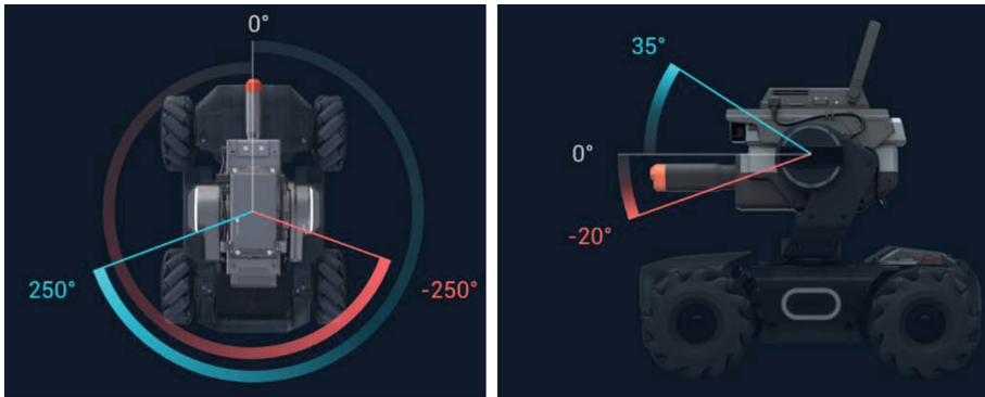
Fig. 7. Illustration from the booklet showing how the gimbal cannon can rotate in pitch and yaw axis.
