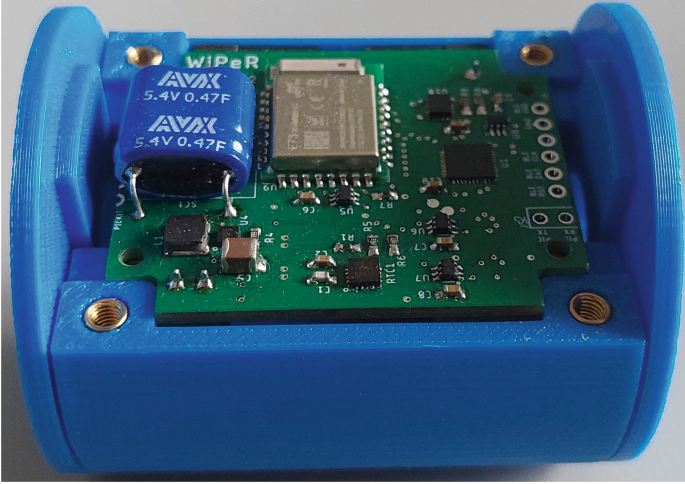
Fig. 5. Device for monitoring bearing faults implementing the FaultBit toolkit
