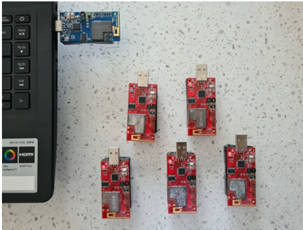
Fig. 4. The hardware used for the experiment with one telosB mote connected to the notebook for data collection
