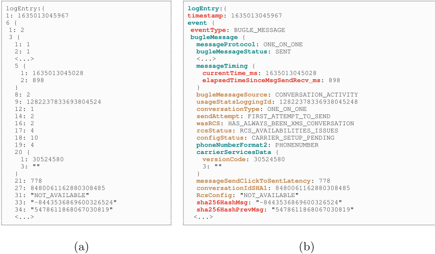
Fig. 4. Example of Google Messages ANDROID_MESSAGING Clearcut logger log entry: (a) protobuf decoded using Google Protobuf compiler with the --decode_raw option, (b) after reverse engineering the schema.
