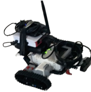
Fig. 1. Mobile NXT robot with a mounted Raspberry Pi 3.
