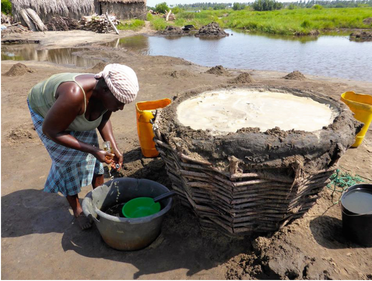
Fig. 2. Traditional filter composed of a first layer of braided mangrove branches, then a second layer of thin clothing superimposed as a filter, into which the salted sand crust and the lagoon water are poured. The filter also has a pipe at the base to collect the brine (source: Nouvelle Afrique Magazine 2018/03/26).
