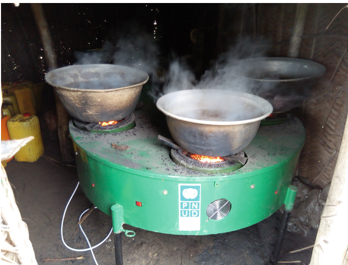
Fig. 5. Mivo stove structure using solar panel as energy source and palm nut hulls.
