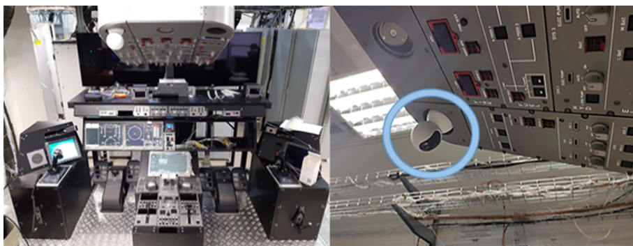
Fig. 3. Avionics integration bench and webcam mounted on it
