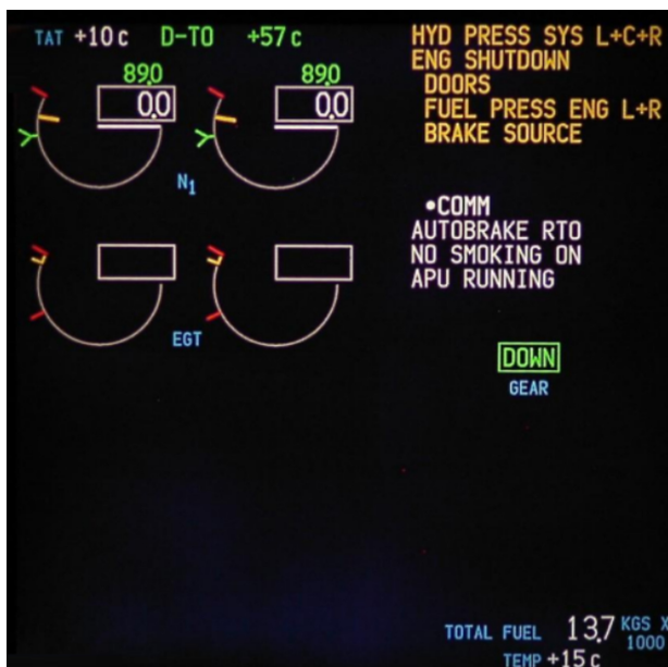
Fig. 2. The Boeing 777 EWD example [5].
