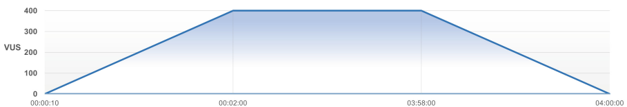
Fig. 11. Soak testing - VUs progress over time
