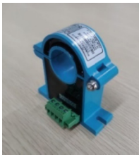
Fig. 3. Mutual inductance current detection sensor
