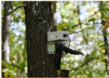
Fig. 3. Air moisture, humidity, and temperature sensor.
