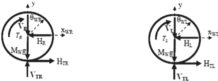
Fig. 3. Force analysis of right and left-wheel [8]
