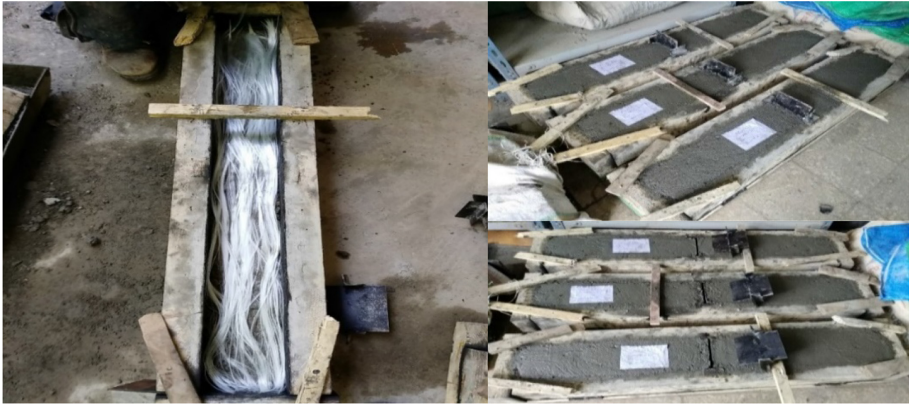
Fig. 4. Glass fiber in layer, casted beam with notch plate & notch plate removed
