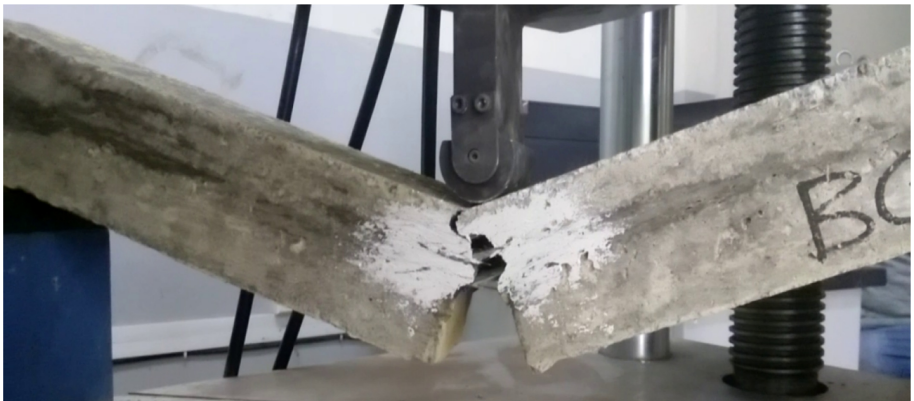
Fig. 14. Crack patterns at 0.6% glass fiber addition for C20/25 design grade concrete just before failure.
