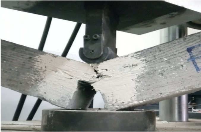
Fig. 11. Crack patterns at 0.6% glass fiber addition for C25/30 design grade concrete.
