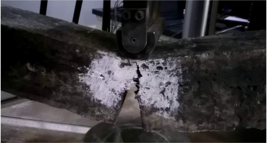
Fig. 13. Crack patterns at 0.4% glass fiber addition for C20/25 design grade concrete just before failure.
