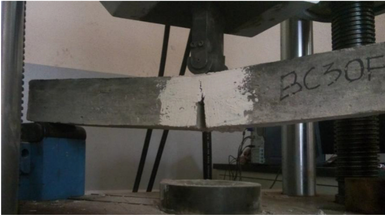
Fig. 9. Crack patterns at 0.2% glass fiber addition for C25/30 design grade concrete just before failure.
