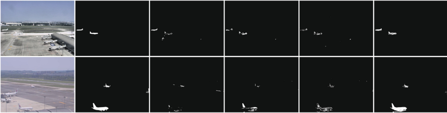
Fig. 5. Left to right: two frames in S12 and S20 , ground truth, SOBS [15], PBAS [14], CodeBook [11] and the proposed method, respectively.
