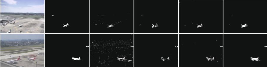
Fig. 4. Left to right: two frames in S1 and S21 , ground truth, KDE [12], KNN [10], Bodids [6] and the proposed method, respectively.
