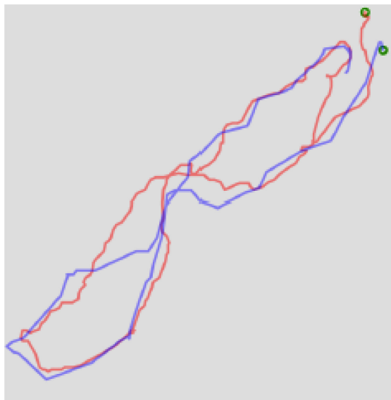
Fig. 8. Result obtained with the GPS for two people walking inside the garden. The blue line is related to the cloud processing and the red line to the custom developed processing. (Color figure online)
