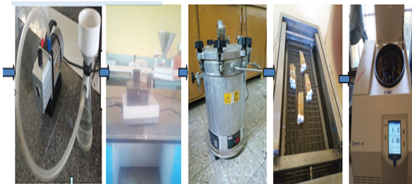
Fig. 2. Alkaline pretreatment and hydrolysis equipment setup
