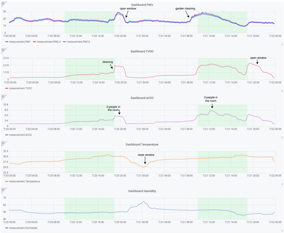
Fig. 5. Data obtained during a 48 h period in a regularly occupied classroom. The plots are annotated with relevant events, such as window state, outdoor events, number of people in the room and cleanings.
