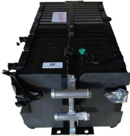
Fig. 1. LiFePO4 battery, used in the project
