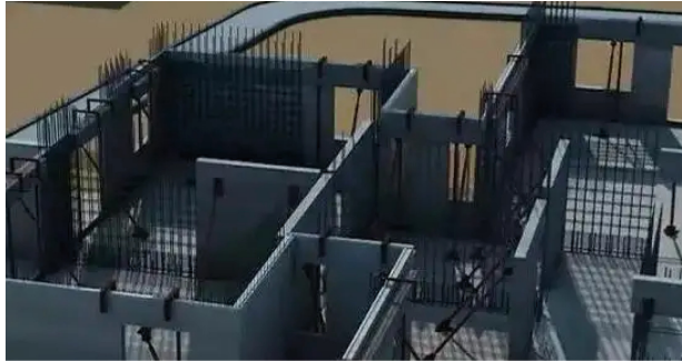
(b) After splicing of prefabricated buildings
