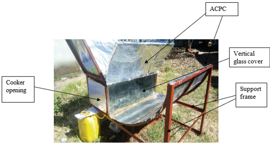
Fig. 2. The manufactured solar cooker on test
