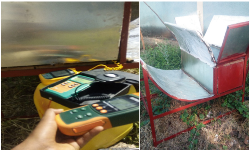
Fig. 3. Experimental setup of the box cooker
