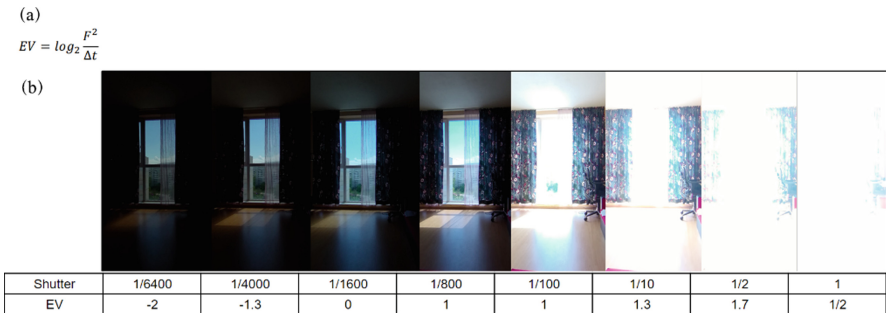
Fig. 1. (a) A measurement of exposure value (EV). (b) Images captures with QooCam8K with different EV and shutter speed.
