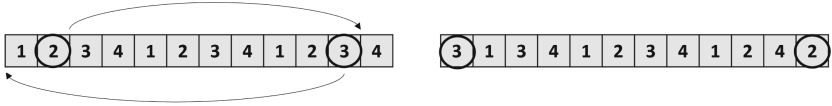
(a) Move the first occurrence of the drone with the highest relative reduction of the mission time, let d_2 , to the tail of the list, and move the last occurrence of the drone with the lowest relative reduction, let d_3 , to the head of the list.
