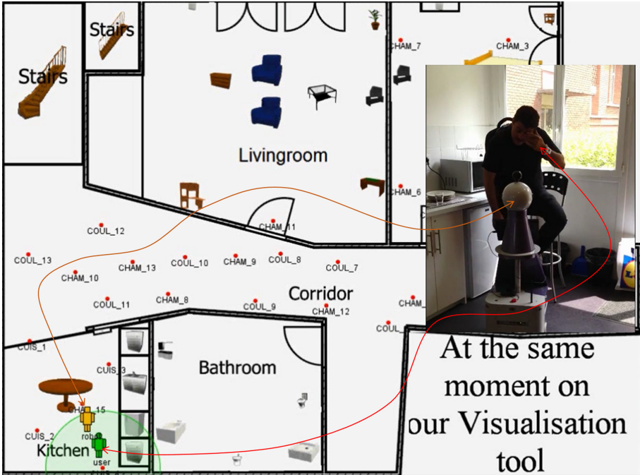
Fig. 2. Depending on the knowledge analysis, The robot accomplishes tasks under different environmental conditions and recognizes situations/contexts. Moreover, distributed IoT devices assist the robot in localizing John. In fact, a concept defined in an ontology becomes identifiable from the data provided by the sensors.
