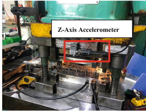
Fig. 2. On-Site Sensor Installation Diagram
