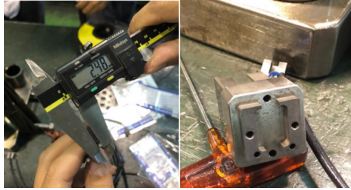
Fig. 9. Illustrates the schematic diagrams of the punch head dimensions, with the left diagram depicting the circular punch head for punching, and the right diagram representing the concave-shaped appearance punch head.
