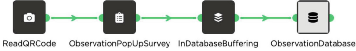
Fig. 5. Application flow graph showing the BufferObservation connecting to ObservationDatabase component on the server-side.
