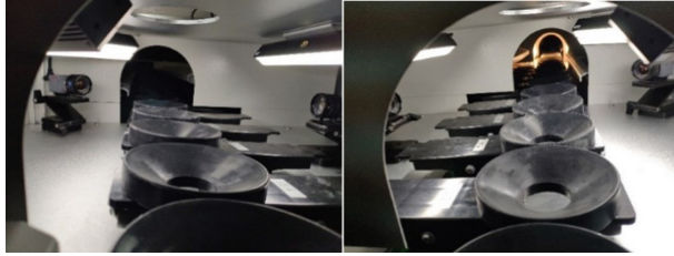
Fig. 2. Apple image acquisition system
