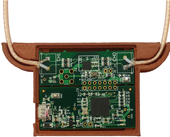
Fig. 3. Inductance Sensor consisting of the evaluation module LDC1612 EVM with two SMA-connectors mounted in a housing.
