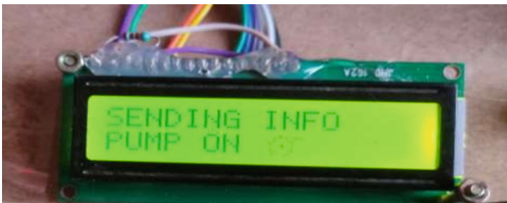
Fig. 6. LCD display of output for sending SMS alerts
