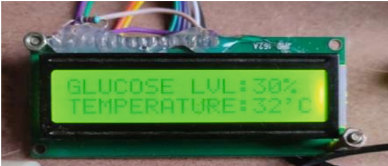
Fig. 5. LCD display of output demonstrating glucose and temperature levels
