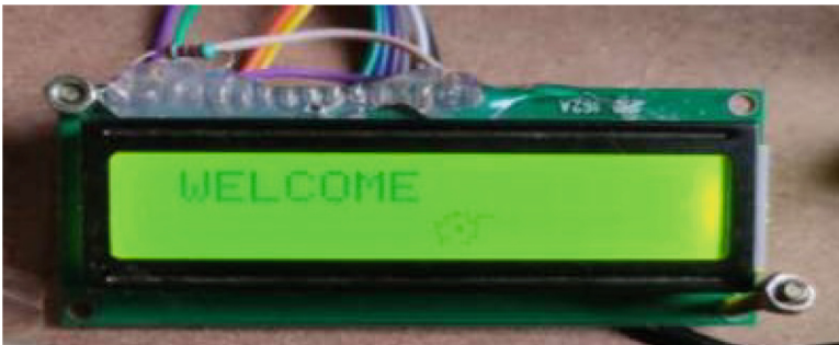
Fig. 4. Initial condition of booting modem on LCD display
