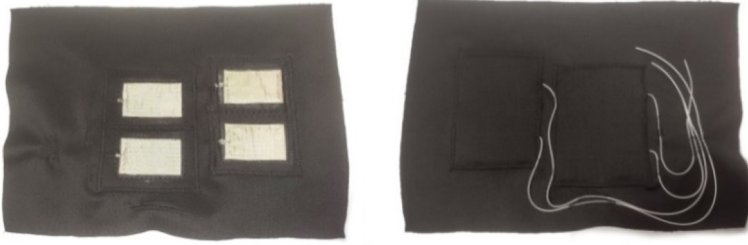
Fig. 3. Electrodes placement on the base fabric: front and back view
