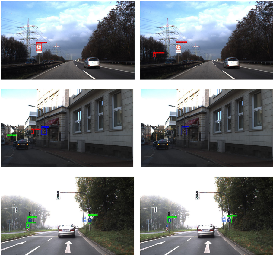
Fig. 6. The detection results of YOLO-RFB (left) and YOLO V4 (right) in GTSDDB
