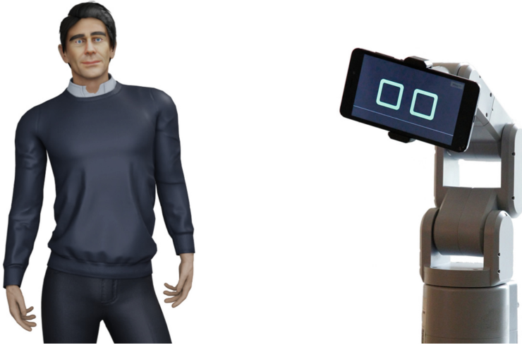
Fig. 1. Virtual Human and Social Robot. The image depicts the life size virtual human (left) while idling and the one-arm robot based social robot (right) during the “Seek Attention” animation.
