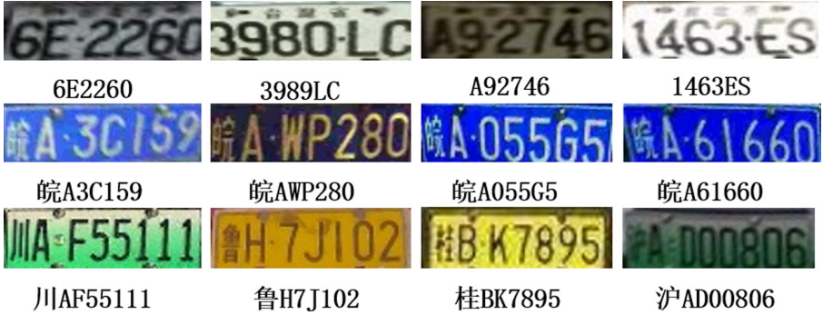
Fig. 5. Rectification LPs from Fig. 4 and recognition results. First line LPs is scale in width for a better view.
