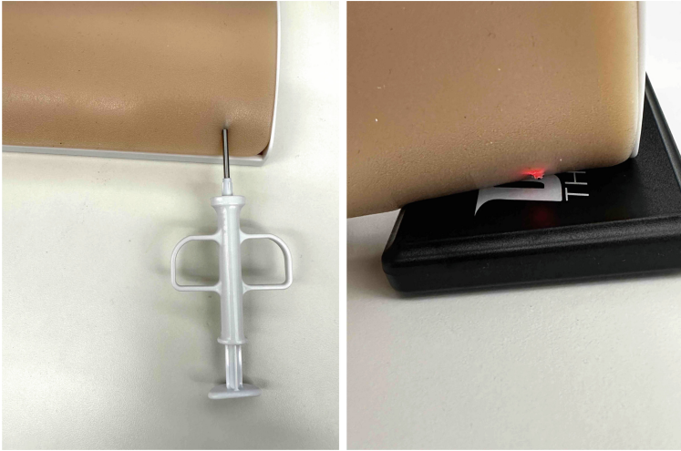
Fig. 4. Injecting the xSSID Implant Into Synthetic Skin and Scanning the Implant From Within the Skin.
