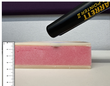
Fig. 7. Testing The flexEM T5577 Implant Being Embedded at Different Depths.
