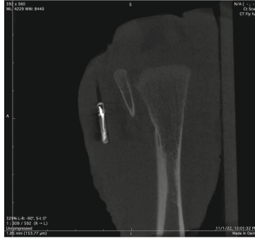
Fig. 5. An X-Ray of an xSIID Implant Within a Bone-in Chicken Thigh.
