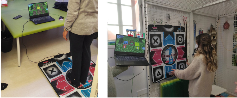
Fig. 1. Physiotherapists testing the prototypes and exploring the mat in different ways, using: (left) lower limbs; (right) upper limbs.
