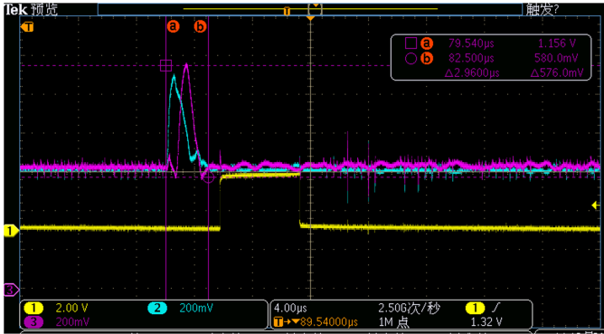
Fig. 7. DCOC settling process (The blue and pink lines represent I-Path and Q-Path DC offset respectively). (Color figure online)
