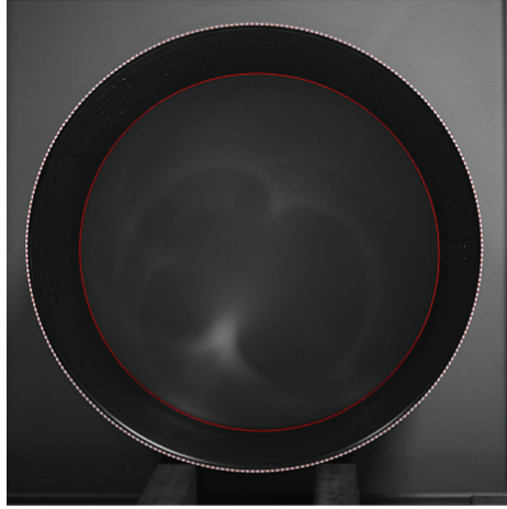
Fig. 4. An image of the cylinder from top with extracted edges (Courtesy of BLINDED).
