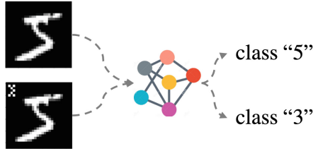
Fig. 2. In the inference phase, the backdoored model for handwritten digital image classification correctly classifies benign inputs as class “5” while classifying malicious inputs into a predefined target class “3”.
