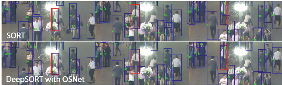
Fig. 6. Frames from MOT17 [18]. Top row are results using SORT [25], bottom row – using VSF [1] (DeepSORT [10] and OSNet [9]). VSF correctly identifies the pedestrian in red rectangle with an identity 3, whereas SORT incorrectly assigns him three different identities – 48, 65, 75.
