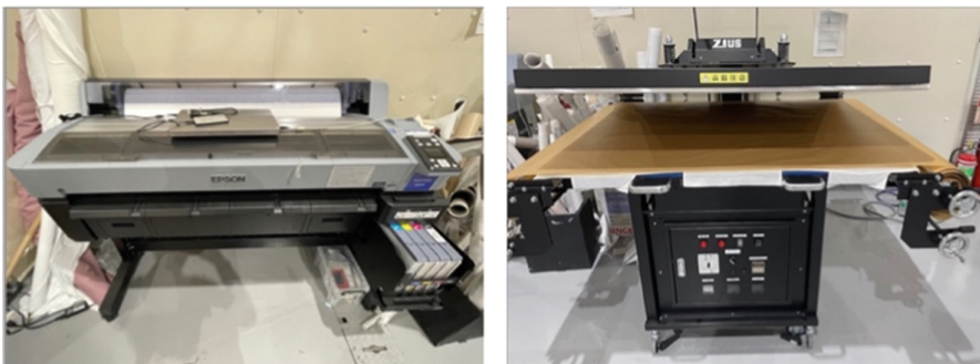
Fig. 4. Inkjet printer for sublimation transfer (left) and thermal transfer device (right).
