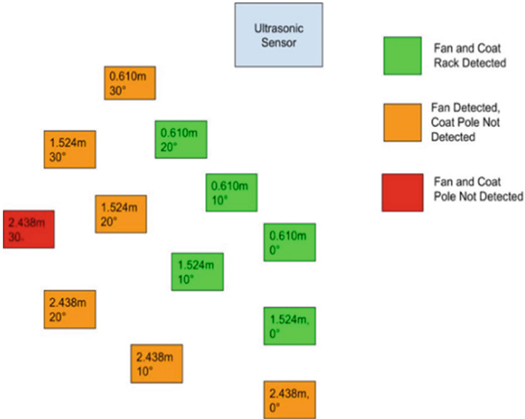
Fig. 7. Location of Obstacle Detection, the green box locations mark places where both the pole (narrow diameter) and fan (wide diameter) were consistently detected, the yellow box locations mark places where the pole was not consistently detected, but the fan still was, and the red box marks a spot where neither the pole nor the fan was consistently detected. (Color figure online)
