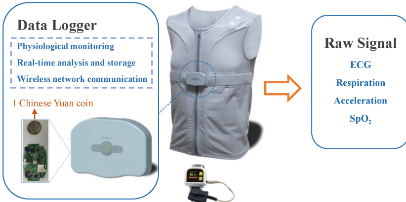
Fig. 2. Hardware and signal acquisition of SensEcho.
