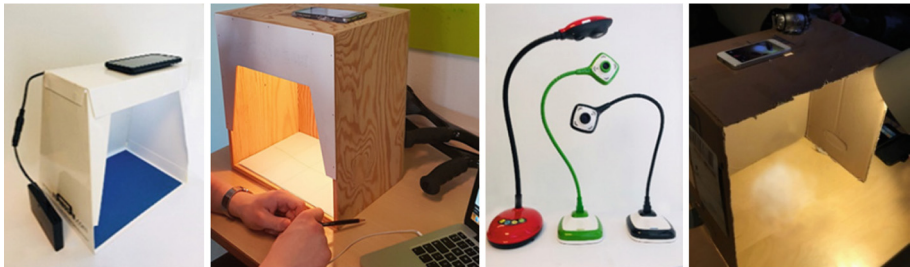
Fig. 6. The first image depicts a lightbox made of cardboard called a “standscan.” The second image depicts a lightbox made in wood developed by one of our master’s students. The third image depicts a flexible cable camera in which the “neck” of the camera can be shaped, allowing for a change in perspective. The last photo depicts a lightbox created from a regular cardboard box utilizing bicycle lights.
