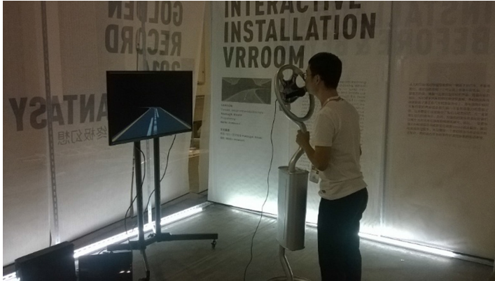
Fig. 3. Interacting with the road in virtual environment and controlling movement by making sound of car engine and modulating its intensity. (© Predrag K. Nikolic. Photo: Predrag K. Nikolic)
