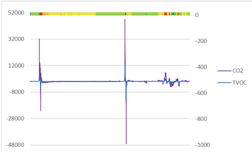
Fig. 8. Plots of the CO 2 and TVOC derivatives values for the second test. The vertical black lines (at the bottom) mark the moments where events have occurred. Also shown by the horizontal colored bar is the color produced by the light LED corresponding to the forecasting of the indoor air quality index (green—Excellent, light green—Good, yellow—Moderate, orange—Poor, and red—Unhealthy). As can be seen, the predicted values are in line with the measured ones (Fig. 7). (Color figure online)
