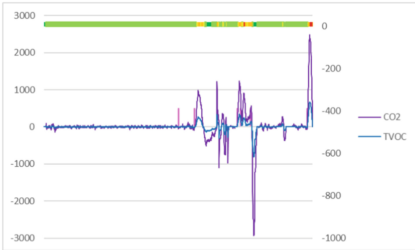
Fig. 6. Plots of the CO 2 and TVOC derivatives values for the first test (please refer to the main text). The vertical black lines (at the bottom) mark the moments where the events have occurred. Also shown by the horizontal colored bar is the color produced by the light LED corresponding to the forecasting of the indoor air quality index (green—Excellent, light green—Good, yellow—Moderate, orange—Poor, and red—Unhealthy). As can be seen, the predicted values are in line with the measured ones (Fig. 5), being, as expected, more severe at the moments where the air quality changes abruptly. (Color figure online)
