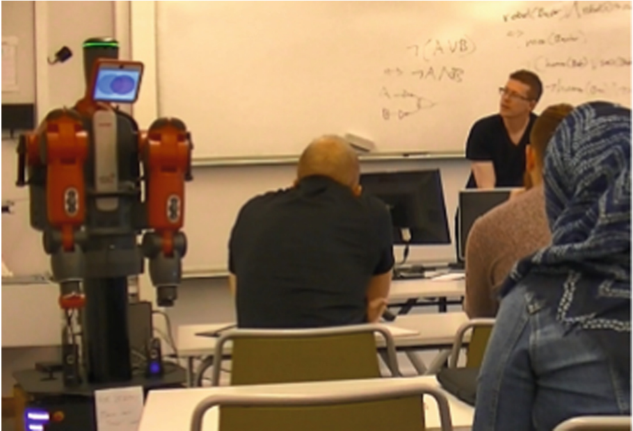
Fig. 2. Displayer. A Baxter robot displays words that a teacher speaks during a class on its small display screen.
