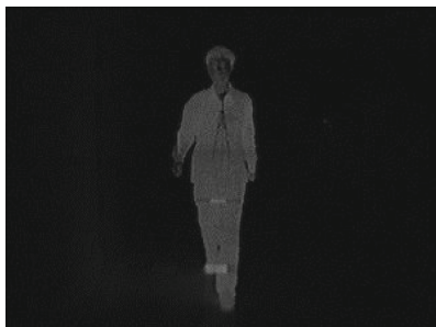
Fig. 3. Image obtained by background subtraction method
