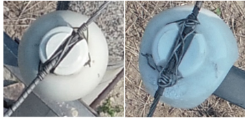
Fig. 7. Image comparison of intact and damaged porcelain bottles
