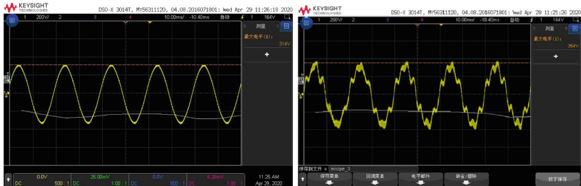
Fig. 5. The voltage waveform when one inverter is connected to the grid and the voltage waveform when two inverters are connected to the grid
